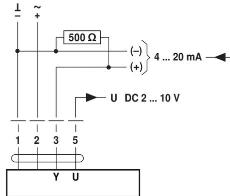
The 500 Ω resistor converts the 4 ... 20 mA current signal to a voltage signal DC 2 ... 10 V
