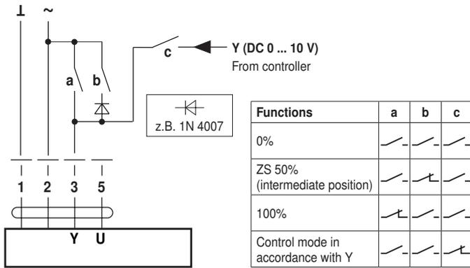
Override control with AC 24 V with rotary control switch
