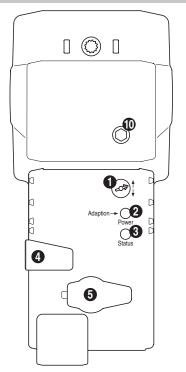
(1) Direction of stroke switch Switching: Direction of stroke changes
