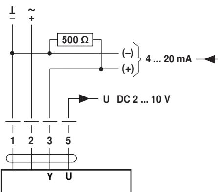
The 500 Ω resistor converts the 4 ... 20 mA current signal to a voltage signal DC 2 ... 10 V
