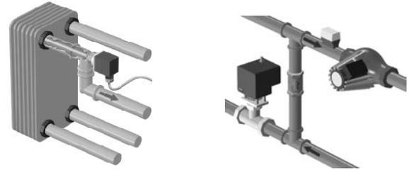
Make sure that the surface of the pipe is clean and even where the sensor is mounted.
