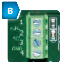
6 Screw terminals Active output signals 0 – 10 V, 4...20 mA, or switching outputs.
