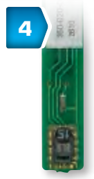
4 Digital humidity and temperature sensor Highly precise, long-term stable, and temperature-compensated.
