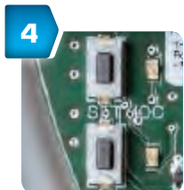
4 Trigger for CO 2 or VOC zero point
