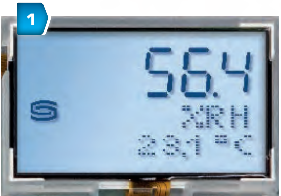
1 Extra-large display (70 x 40 mm) with backlighting, displaying range violations and physical units.
