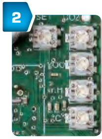
2 Potentiometer - for setting the relay switching thresholds for CO 2 /VOC - for setting the offset for temperature, humidity, CO 2 , VOC
