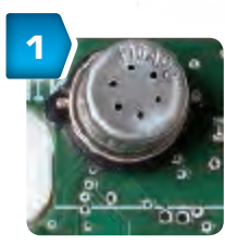
1 Mixed gas sensor (VOC) Air quality sensor
