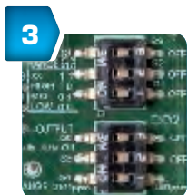
3 DIP switches for individual adjustment of measuring ranges, output, automatic zero point and relay assignment.
