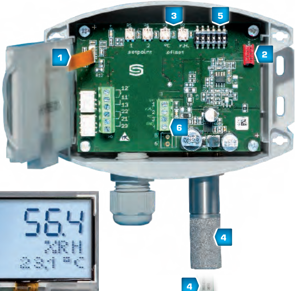
1 Extra-large display (70 x 40 mm) with backlighting, displaying range violations and physical units.
