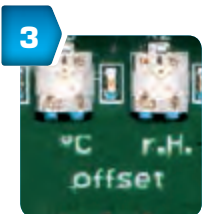
3 Offset potentiometer For fine adjustment (zero point offset), for readjustment, for recalibration.
