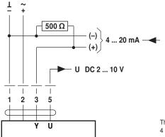
The 500  $\Omega$  resistor converts the 4 ... 20 mA current signal into a voltage signal DC 2 ... 10 V
