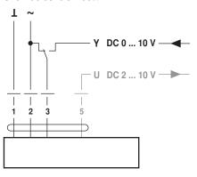
A typical use for 100% override control is in a frost protection circuit. Whether or not the frost thermostat has to interrupt the signal conductor to the controller «d» depends on the make of controller being used (not necessary, if the signal output at the controller is short circuit proof and protected against polarity reversal).
