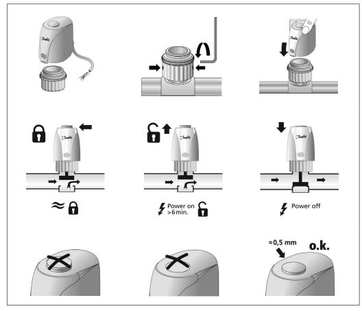
ABNM can be mounted in 360°. Due to high IP class moist is not a problem. A 2 mm Allen key is used to fit valve adapter.
