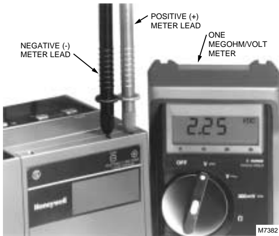
Fig. 11. Measuring flame signal voltage of 7800 SERIES controls.
